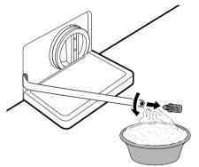
4 Unscrew the drain pump filter slowly to drain the remaining water and then proceed to remove any debris or objects from the filter.
